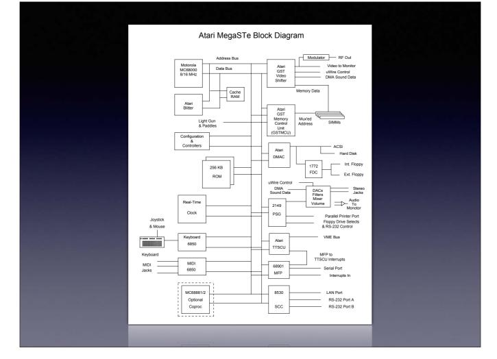
Block diagram of an Atari ST variant Note how everything is connected by three buses— the address bus, data bus, Also a clock to keep everything in sync...
