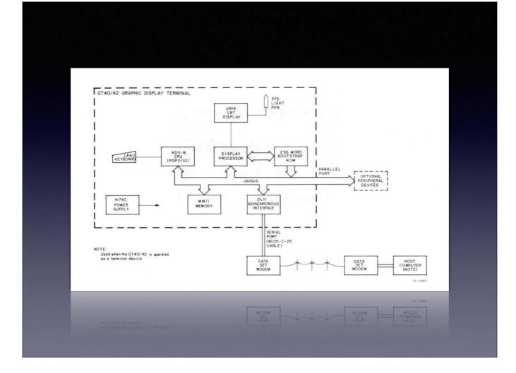
DEC GT40 has a 'unibus' but if we look deeper we can see it is made up of an address, data and control bus...
